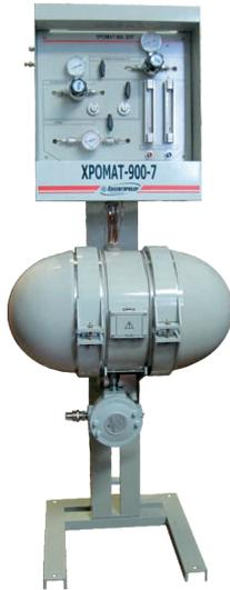
Designed for continuous automatic measuring of mole fraction of nitrogen, oxygen, carbon dioxide, hydrocarbons C1 – C5 and C6 + higher contained in flammable natural gas according to ГОСТ 31371.7-2008 "Natural gas. Determination of composition with defined uncertainty by gas chromatography method. Measurement procedure of the mole fraction of components".
